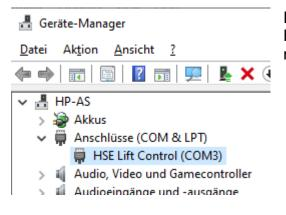
Driver installation was successfull if the main board HSE is displayed here. The displayed COM port may vary.
